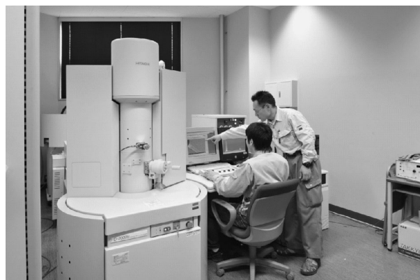
写真-1 走査型透過電子顕微鏡 STEM (Scanning Transmission Electron Microscopy)
